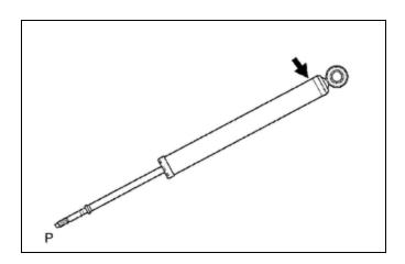
(b) Using a hacksaw, slowly make a hole at the position indicated by the arrow in the illustration to discharge the gas inside.
