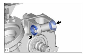
(b) If the bushings are deformed, missing or damaged, replace the electric power steering column sub-assembly with a new one.
