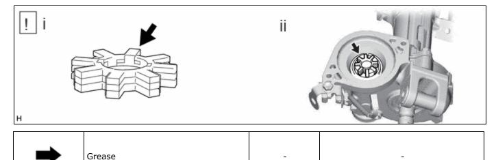
(1) Apply grease to a new electric power steering motor shaft damper.
