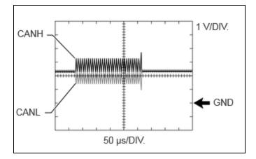
(2) Open in both of the lines (CANH and CANL) of a CAN branch
