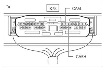
\*a Component with harness connected (Central Gateway ECU (Network Gateway ECU))
