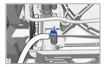
(e) Loosen the drain cock plug indicated in the illustration and drain the coolant.
