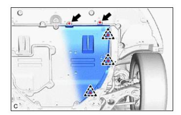
(c) Pull down the No. 1 engine under cover assembly.
