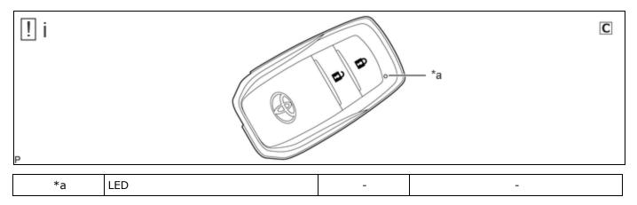
(1) Press one of the transmitter switches and check that the LED illuminates.
