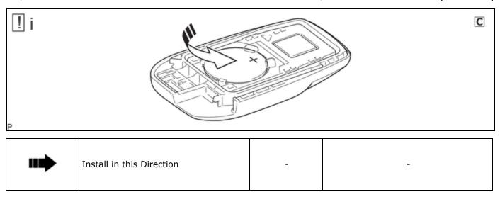
(1) Install the transmitter battery (lithium battery: CR2450) with the positive (+) side facing upward, as shown in the illustration.
