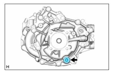
(d) Using a 10 mm hexagon socket wrench, install a new gasket and the drain plug to the rear traction motor with transaxle assembly.
