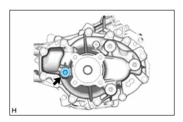
(c) Using a 10 mm hexagon socket wrench, remove the drain plug and gasket from the rear traction motor with transaxle assembly and drain the hybrid transaxle fluid.
