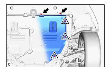
(b) Pull down the No. 1 engine under cover assembly.
