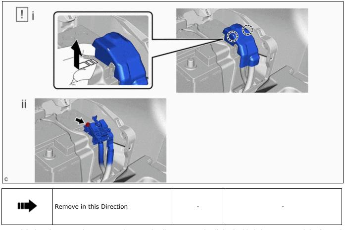
(1) Place fingers on the positions shown in the illustration and pull the fusible link cover toward the front of the vehicle to disengage the claw and remove the fusible link cover.
