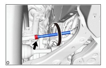
(c) Turn the right and left steering rack ends by an equal amount to adjust the toe-in.
