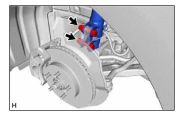
(c) Remove the top and bottom bolts one at a time and confirm that the steering knuckle can move freely in the front shock absorber assembly.
