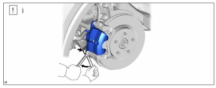
(1) Hold the front disc brake cylinder slide pin (lower side) and remove the bolt.
