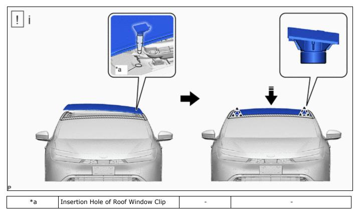
(1) Install the No. 1 roof window glass sub-assembly.
