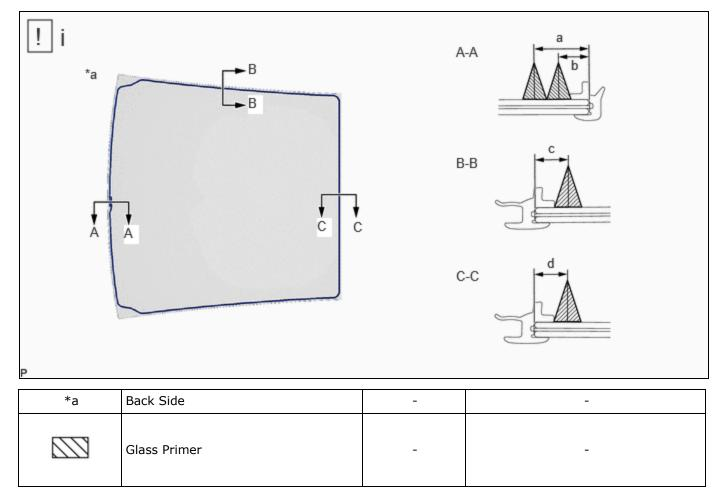
(1) Apply adhesive to the No. 1 roof window glass sub-assembly as shown in the illustration.
