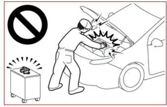
• After removing the service plug grip, wait for at least 10 minutes before touching any of the high-voltage connectors or terminals.
