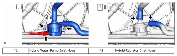
(1) Disconnect the inverter water pump with motor assembly connector.
