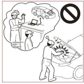
• To reduce the risk of electric shock, do not perform troubleshooting before checking for DTCs.
