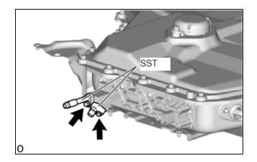
(c) Connect a refrigerant recovery unit to the SST.
