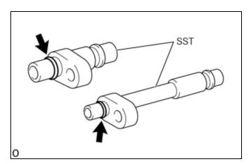
(b) Install the SST with the 2 bolts.
