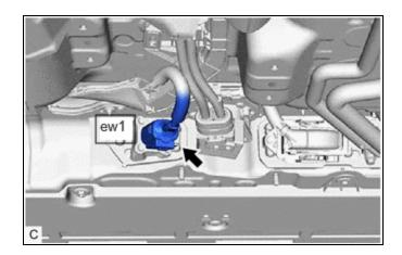
(c) Disconnect the floor under wire connector.
