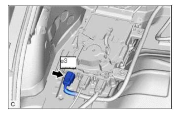
(c) Disconnect the electric vehicle charger assembly connector.
