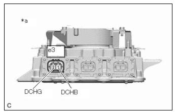
\*a Component without harness connected (Electric Vehicle Charger Assembly)
