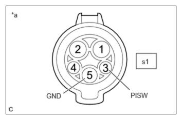
\*a AC Charger Inlet Cable (Charging Inlet)
