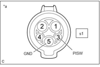
\*a AC Charger Inlet Cable (Charging Inlet)
