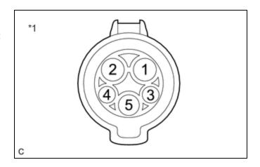
\*1 Inlet AC Charger Cable (Charging Inlet Side)
