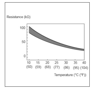
The resistance of the thermistor built into the generator temperature sensor changes in accordance with changes in generator (MG1) temperature. The lower the generator (MG1) temperature, the higher the thermistor resistance. Conversely, the higher the generator (MG1) temperature, the lower the resistance.
