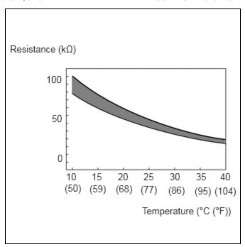
The resistance of the thermistor built into the motor temperature sensor changes in accordance with changes in the motor (MG2) temperature. The lower the motor (MG2) temperature, the higher the thermistor resistance. Conversely, the higher the motor (MG2) temperature, the lower the resistance.
