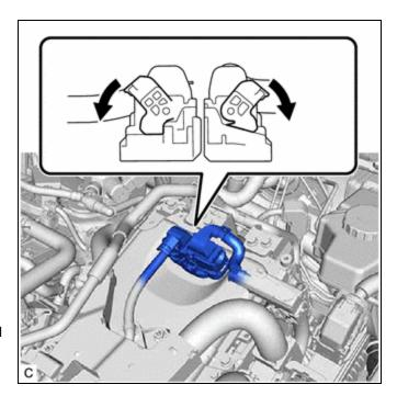
click will be heard as its claw engages. After the click is heard, pull up on the connector to confirm that it is securely connected.
