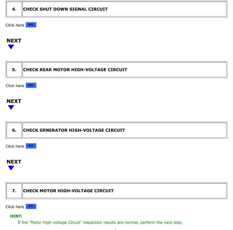
NEXT > REPLACE INVERTER WITH CONVERTER ASSEMBLY
