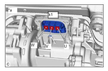
\*a HV floor under wire (rear traction motor cable) not connected (Rear Traction Motor with Transaxle Assembly)
