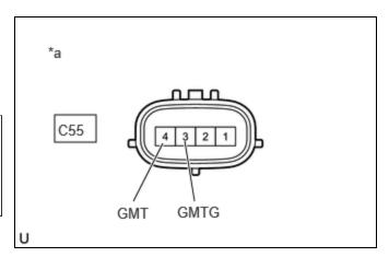
\*a (Generator Temperature Sensor (Hybrid Vehicle Transaxle Assembly))
