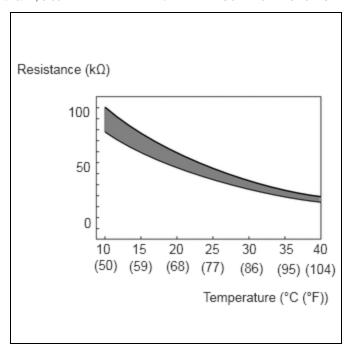
The resistance of the thermistor built into the generator temperature sensor changes in accordance with changes in generator (MG1) temperature. The lower the generator (MG1) temperature, the higher the thermistor resistance. Conversely, the higher the generator (MG1) temperature, the lower the resistance.
