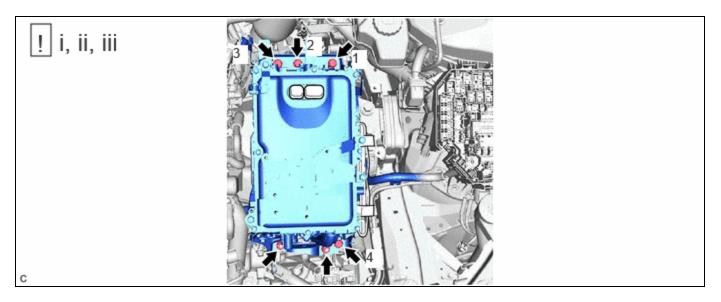
(1) Temporarily install the inverter with converter assembly with the 4 bolts and 2 nuts.
