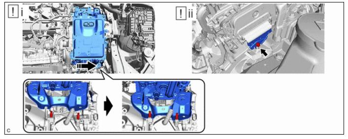
(1) Shift the position of the inverter with converter assembly and temporarily set it on the hybrid vehicle transaxle assembly as shown in the illustration.
