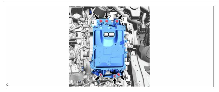
(1) Temporarily install the inverter with converter assembly with the 5 bolts and 2 nuts.
