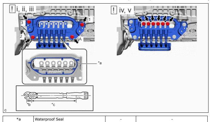
(1) Temporarily install the motor cable to the inverter with converter assembly with the 4 bolts,
