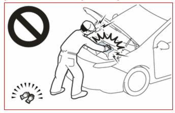
• To prevent electric shock, make sure to remove the service plug grip to cut off the high voltage circuit before
