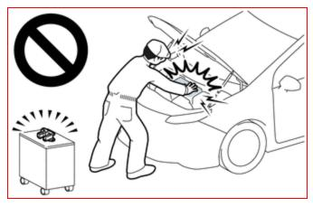
• After removing the service plug grip, wait for at least 10 minutes before touching any of the high-voltage connectors or terminals.
