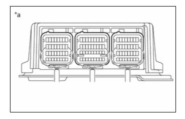
\*a Component with harness connected (Airbag ECU Assembly)
