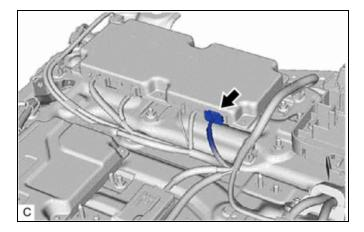
(c) Disconnect the No. 1 traction battery device box assembly connector.
