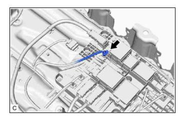
(d) Disconnect the HV battery high voltage connectors from the traction battery device box No. 1.
