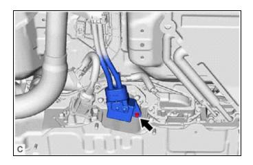
(c) Disconnect the connector from the No. 1 traction battery device box assembly.
