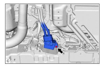
(c) Disconnect the connector from the No. 1 traction battery device box assembly.
