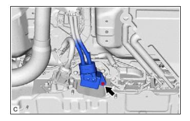
(c) Disconnect the floor under wire connectors from the HV battery junction block assembly.
