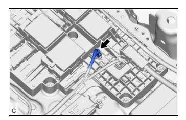
(d) Disconnect the HV battery high voltage connectors from the No. 1 traction battery device box assembly.
