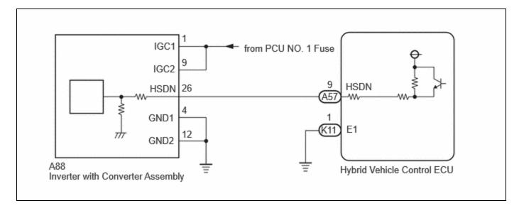
Refer to the wiring diagram for the ECU Power Source Circuit.
