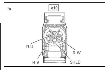
\*a HV Floor Under Wire (Rear Traction Motor Cable)
