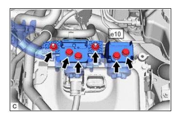
(c) Disconnect the HV floor under wire (rear traction motor cable) from the rear traction motor with transaxle assembly.
