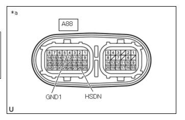
\*a Component without harness connected (Inverter with Converter Assembly)
