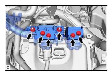
(c) Disconnect the HV floor under wire from the inverter with converter assembly.
