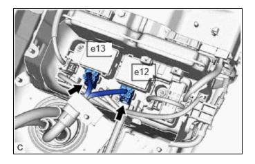
(c) Disconnect the HV floor under wire connectors from the HV battery junction block assembly.
