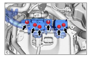
(c) Disconnect the HV floor under wire from the inverter with converter assembly.
