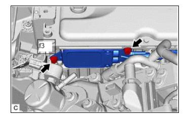
(c) Disconnect the HV air conditioning wire connector from the compressor with motor assembly.
