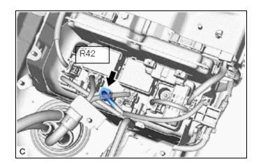
(c) Disconnect the hybrid vehicle control ECU connector.
