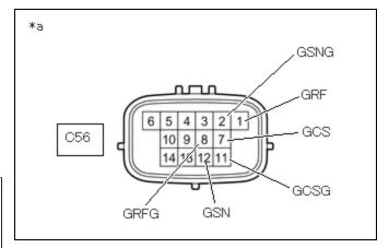
\*a (Generator resolver (Hybrid Vehicle Transaxle Assembly))
