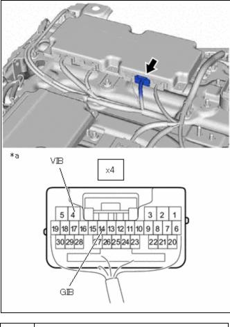
\*a Component with harness connected (Battery ECU Assembly)
