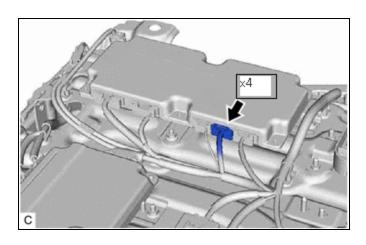
(d) Disconnect the No. 1 traction battery device box assembly connector.
