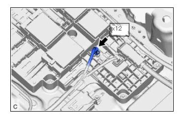
(c) Measure the resistance according to the value(s) in the tables below.
