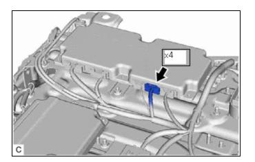
(d) Disconnect the No. 1 traction battery device box assembly connector.
