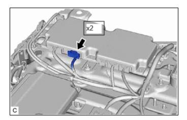
(c) Disconnect the No. 1 traction battery cooler tube connector.
