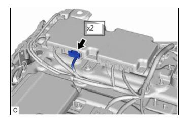
(d) Disconnect the No. 1 traction battery cooler tube connector.
