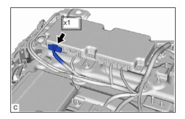
(c) Disconnect the x6 battery voltage sensor connector.
