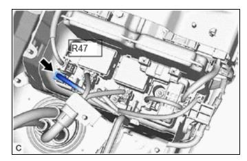
(c) Disconnect the No. 1 traction battery device box connector.
