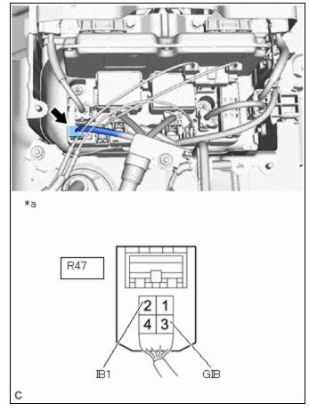
Component with harness connected\*a (No. 1 Traction Battery Device Box (Battery Current Sensor))
