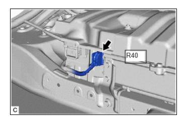
(c) Connect the cable to the negative (-) auxiliary battery terminal.
