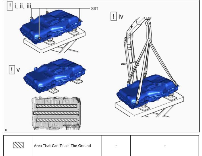
(1) Slowly lower the engine lifter to remove the HV supply battery assembly.
