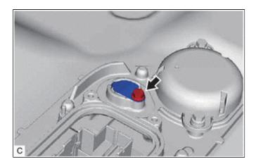
(j) Install SST with the wing bolt as shown in the illustration.
