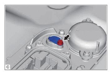
(d) Remove the bolt and cover from the HV supply battery sub-assembly.
