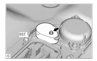
(f) Install SST to the HV supply battery sub-assembly with the 4 bolts.
