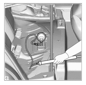
(o) When the gauge pressure reaches 2.0 kPa, close the valve.
