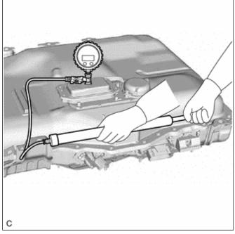
(h) Close the valve, wait 20 minutes, and then check that the gauge pressure has not decreased by more than the specified value.
