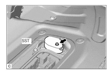
(m) Install SST to the HV supply battery sub-assembly with the 4 bolts.
