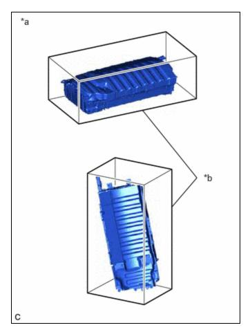
(1) Set the HV battery in the container (A).
