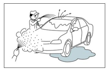
(1) Sprinkle water onto the vehicle and check if the malfunction occurs.
