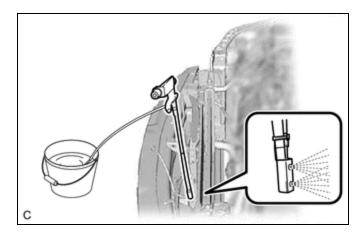
(3) Leave the cooler condenser assembly as is for 10 minutes to let the water penetrate the dirt.
